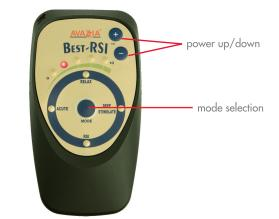
Power levels are accessed by pressing "+" and "-" switches. Simple, easy to see LEDs that indicate different modes and low battery indicator along with automatic shutoff are standard features.
